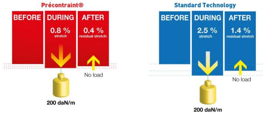
(Deformation test under load)
